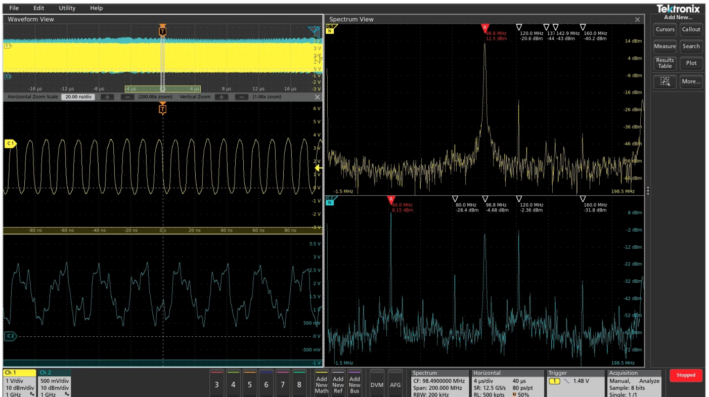
Figure 10: SpectrumView with a Tektronix 4, 5 and 6 Series MSO enables the engineer to look deep into sources of EMI.
