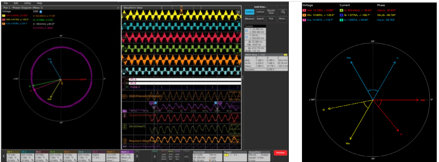
Figure 8: Unique oscilloscope-based phasor diagram feature provides the relation between the voltage and current vectors.
